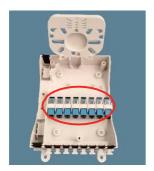
3. Put the fiber to the tray, and let the end in the splicing slot after coiling
