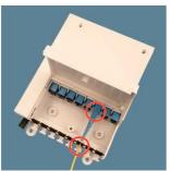
. Strip and clean the cable, keep it 0.8~1.2m long and 30- 50mm long of the strength member, and insert cable through inlet, fix it by cable clamp, and fix strength member by special clamp.
