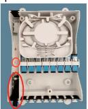
4. Install PLC splitter in the tray, and connect pigtails with adapters, and put the pigtails in the splicing slot, splice with the incoming cables.
